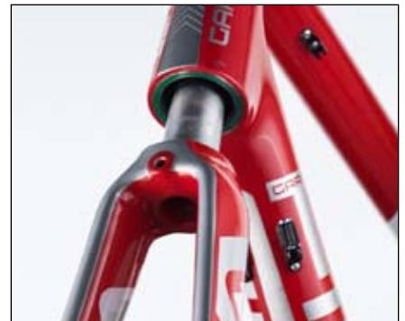
Figure 8. Inserting the fork through the head tube
